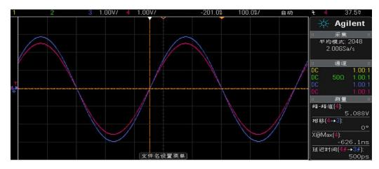
Fig. 3. Display of time delay, 9.4 m versus 0.4 m, at 2.0 MHz
