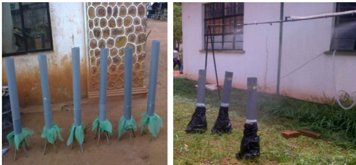
Fig. 3 (a). Constructed leachate extraction columns; (b) simulating rain on the leachate extraction column (source: authors' fieldwork)
