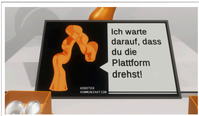
FIGURE 6 | The text panel provided guidance for the current task and an explanation of the robot arms' behavior. The text was displayed within a speech bubble next to a stylized representation of the robot arm to strengthen the affiliation of the statements to the robot arm. The communication was formulated in the first-person form to evoke the perception of the robot arm as a collaboration partner instead of a tool ("I'm waiting for you to turn the platform").
