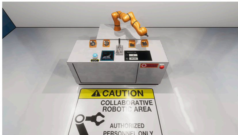
FIGURE 2 | The virtual workplace arrangement at which the participants conducted the shared task in collaboration with the robot arm. Apart from the pin-back button press and the container for the assembly components, the workplace contained a start and emergency shutdown button. Shown is the non-augmented condition where the three communication channels are absent. The virtual workspace where the shared task was executed by the participants in collaboration with the robot arm. The arrangement was designed Note that in the control condition the augmented communication channels are absent.
