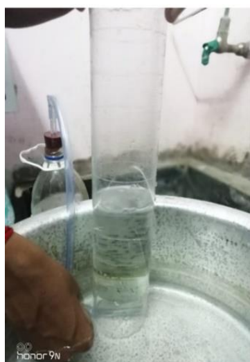
Image 2. Water displacement method – Biogas volume measurement
