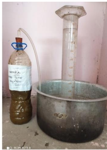
Image 2. Water displacement method – Biogas volume measurement
