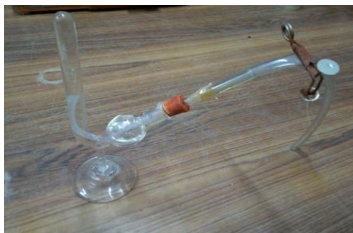
Image 3. Measuring biogas methane content using saccharmeter
