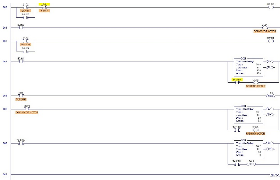
Fig. 5. Ladder logic program for fruit separation and operation the motor
