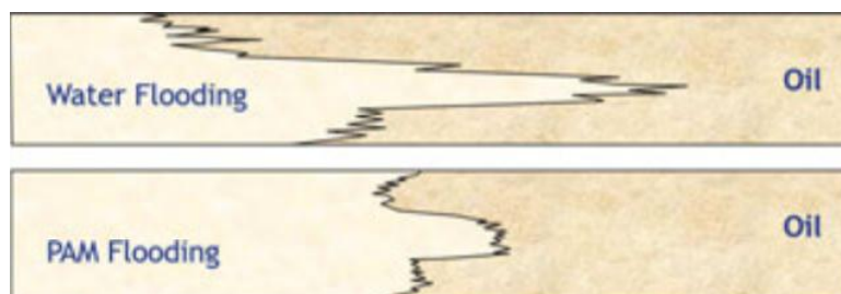
Fig. 2. Water breakthrough delayed and improved sweep efficiency by Polyacrylamide (PAM) polymers (Source, Thomas, [23])
