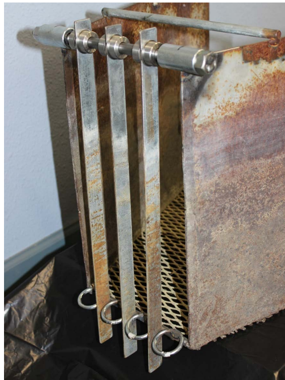
Figure 12. The modified weir after operation during one spawning season.
