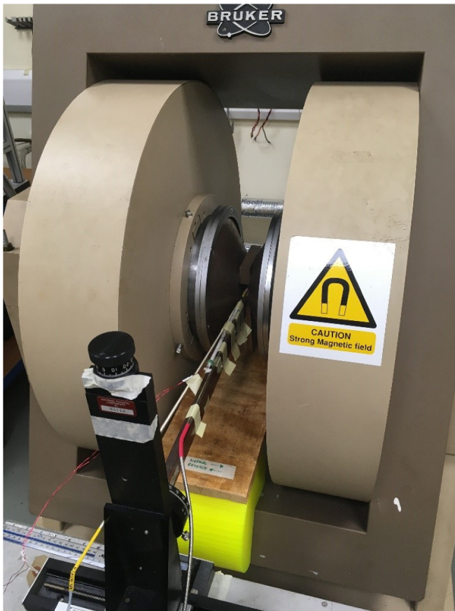
Figure 13. The three probes—NPL phosphor, thermocouple and resistance—mounted between the poles of the Bruker electromagnetic.
