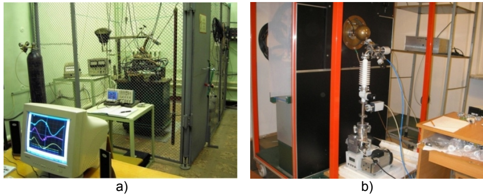
Fig. 2. DPF devices used in these experiments: PF-5M (IMET) (a) and PF-6 (IPPLM) (b)
