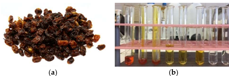
Figure 1. (a) The dried berries from which the oil was isolated, (b) The 8 oils applied in emulsions (from left to right): the commercial Siberian oil, oil extracted in EtOH, oil extracted in hexane, the commercial Greek oil, oil isolated with cold maceration, oil isolated with hot maceration, oil after distillation in H 2 O, sunflower oil.
