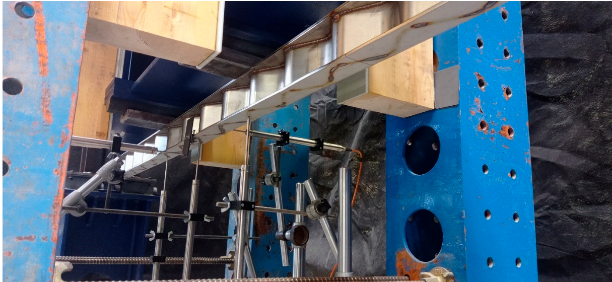
Figure 3. SIN-100 beams: (a) Geometry and the boundary conditions. (b) Cross-section. (c) Experimental test layout.
