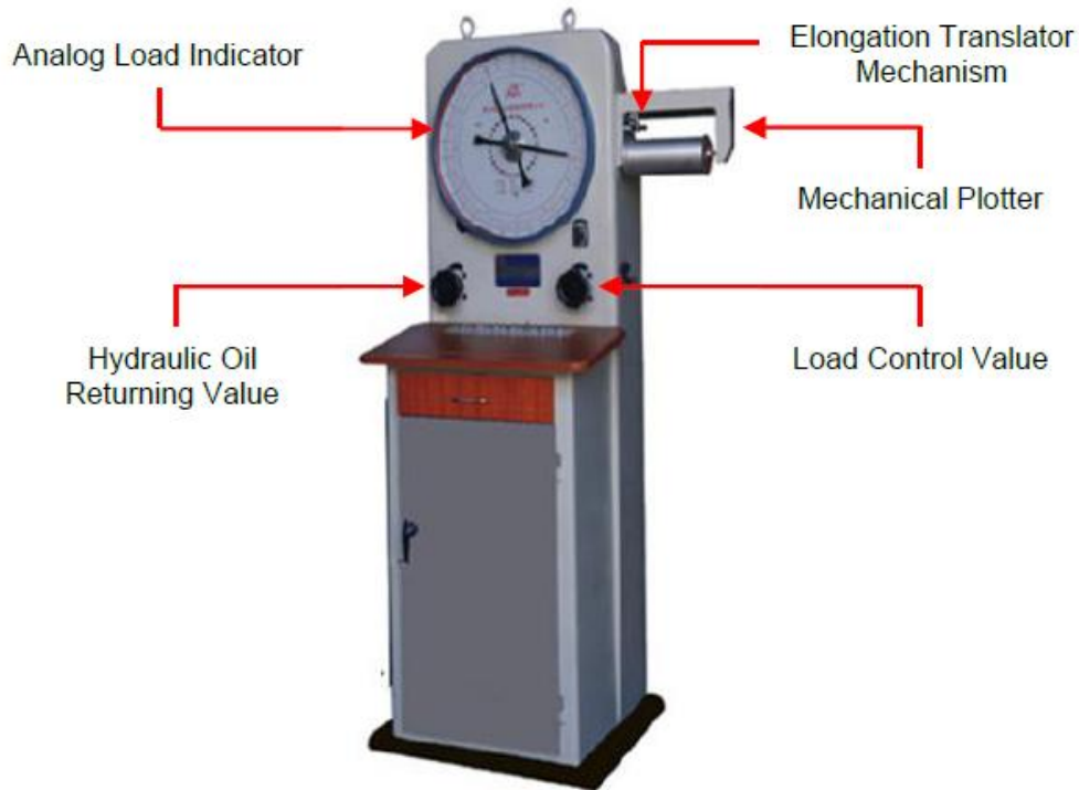
Fig. 3. Control and data acquisition sub-system of analog display type
