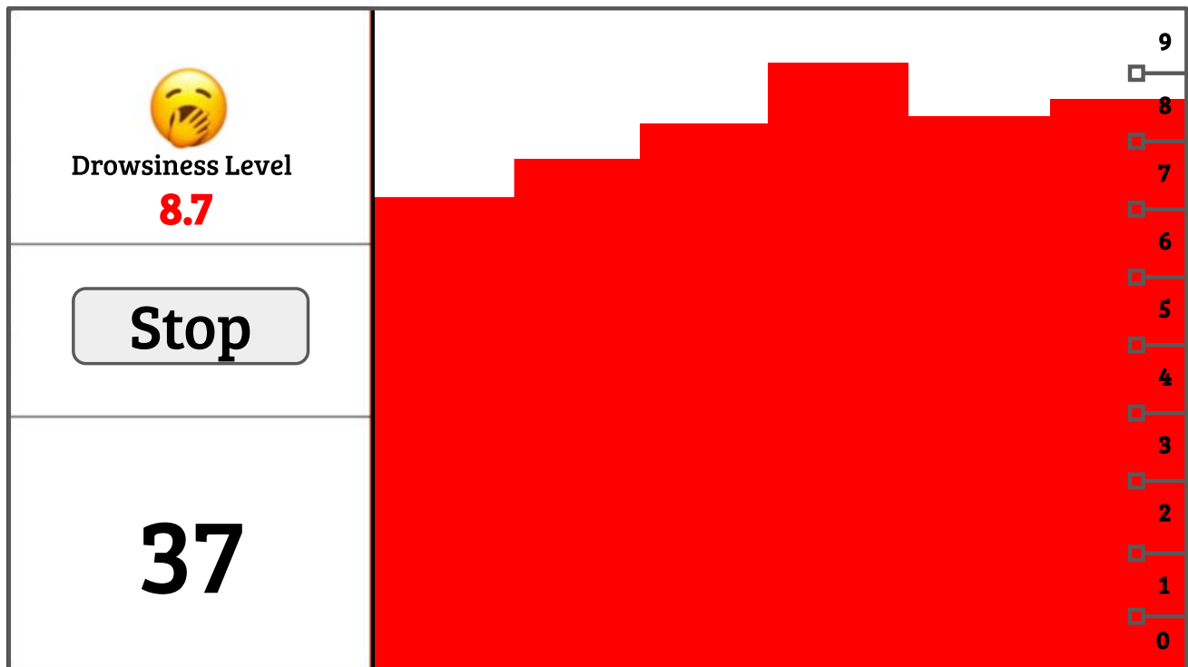
Figure 5. Running example of the user interface. The emoji on the top left describes the current drowsiness status and the bar chart displays on the right the historical drowsiness value over time. On the bottom left, the number of detected blinks is shown so that users can know whether the algorithm is running without error.
