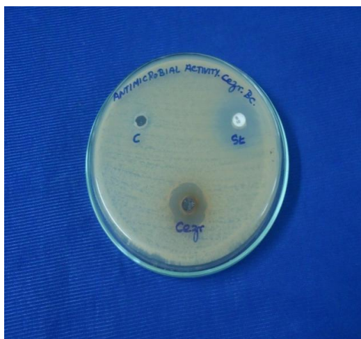
Fig. 7c. Antimicrobial activity of compounds treated against Bacillus sp using by well diffusion method of CeO_2-ZrO_2
