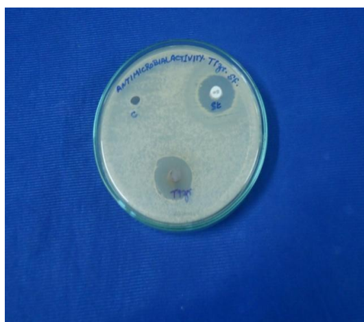
Fig. 7e. Antimicrobial activity of compounds treated against Shigella flexneri using by well diffusion method of TiO_2-ZrO_2
