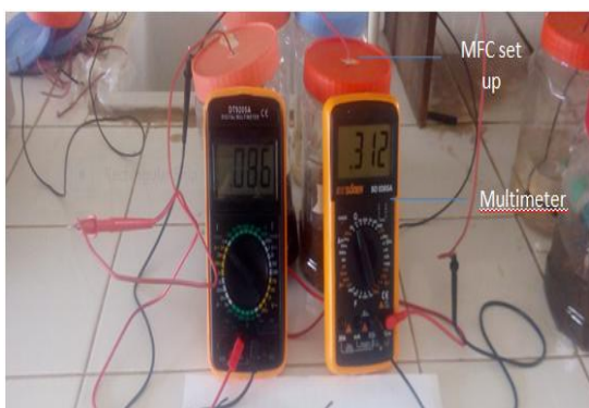
Plate 2. A constructed microbial fuel set up
