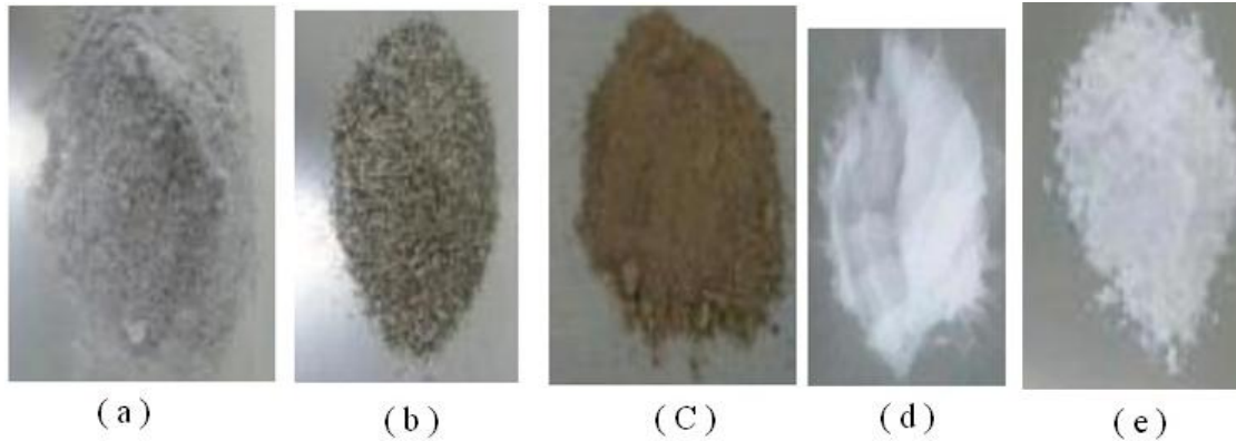
Fig. 2. Different types of dust used in the literature: (a)-Carbonaceous fly-ash, (b)-Sand, (C)-red soil, (d)-silica Gel, (e)-calcium carbonate
