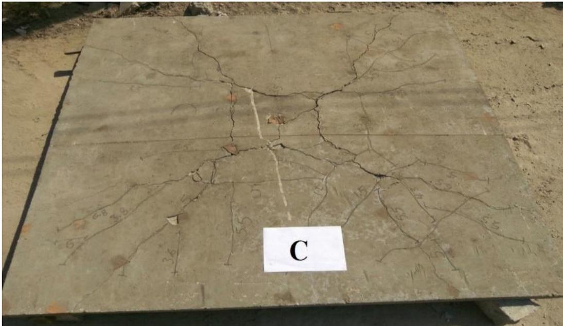
Fig. 18. Cracking pattern of specimen (C)
