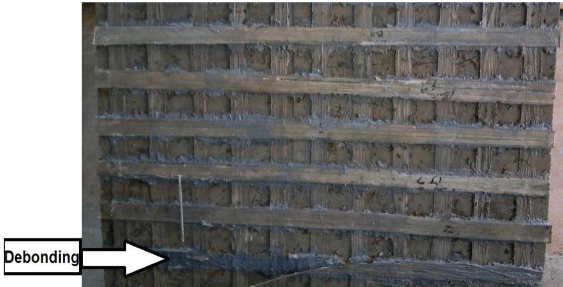
Fig. 20. Debonding shape for specimen (GS-1.5-20-Ag)
