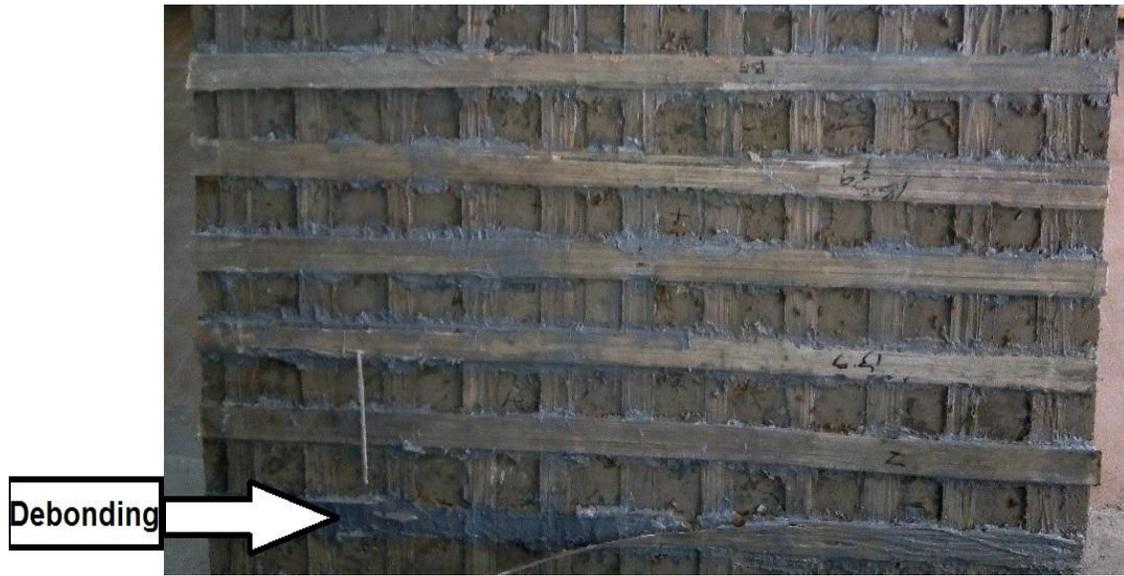
Fig. 20. Debonding shape for specimen (GS-1.5-20-Ag)
