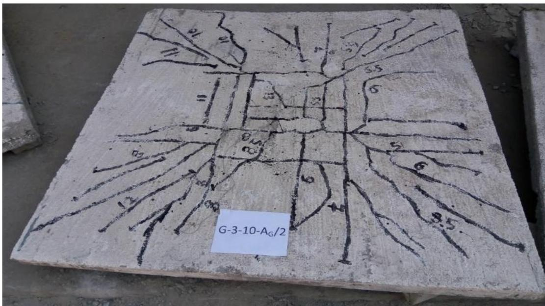
Fig. 19. Cracking pattern of specimen (G-3-10-Ag/2)
